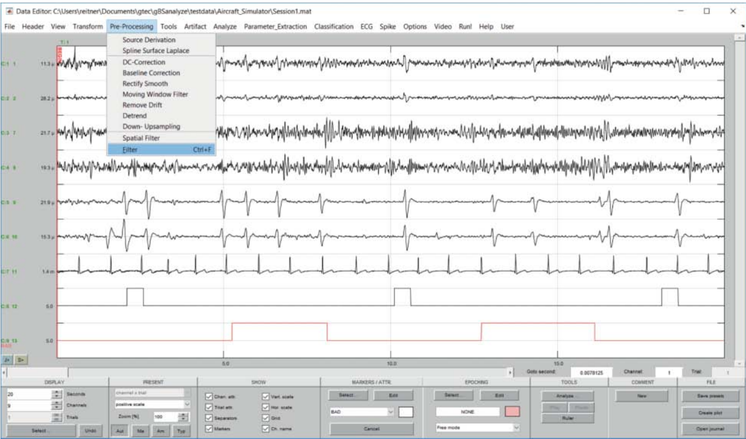
The Data Editor shows the biosignal time series and allows you to scroll through the data. The menu gives access to the analysis functions and every single step is reported in the MATLAB command window.
